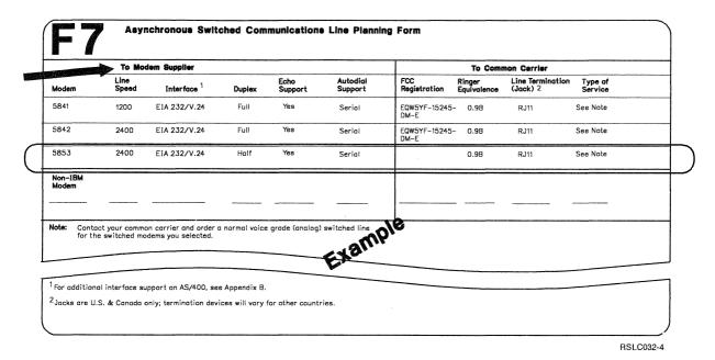
This section of the Asynchronous planning form lists all the IBM modems you could use with this line. Make a choice of which modem suits your needs and circle the entire line that the modem type is recorded on.
